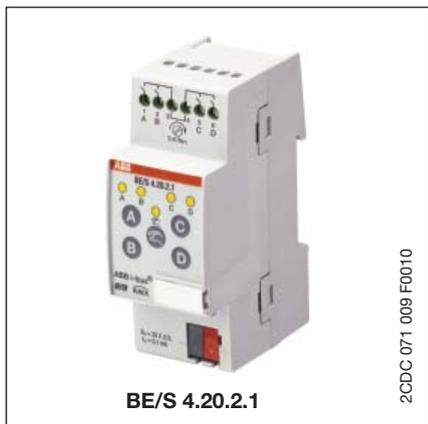
The 4-fold Binary Input BE/S 4.20.2.1 with manual operation is a modular installation device for installation in distribution boards. The device is suitable for detection of floating contacts. The pulsed scanning voltage is generated internally.
