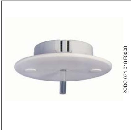
The ABB i-bus® light sensor LF/U 2.1 is a brightness sensor for closed rooms. The light sensor is mounted in a standard installation box in the ceiling. The cover (white) of the sensor is stuck firmly onto the device. The complete unit is then screwed into a flush-type box.
