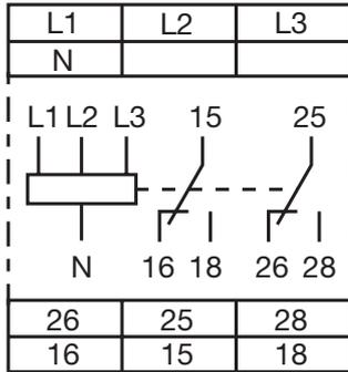
L1, L2, L3, N Control supply voltage = measuring voltage
