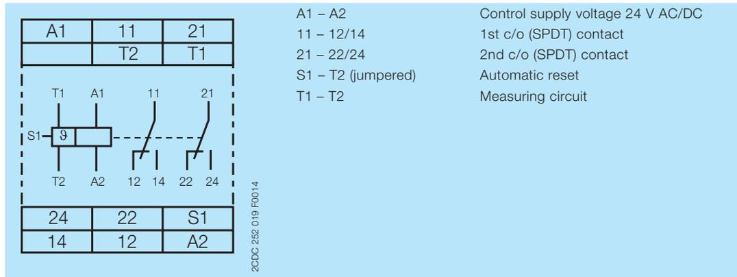
Connection diagram CM-MSS.32
