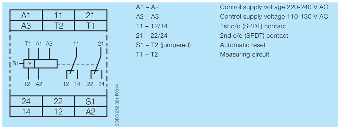
Connection diagram CM-MSS.33
