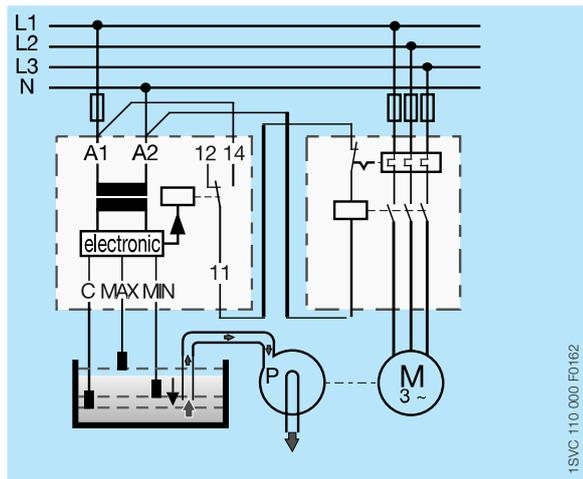
Liquid level control - drain - selected function "↓" (DOWN)
