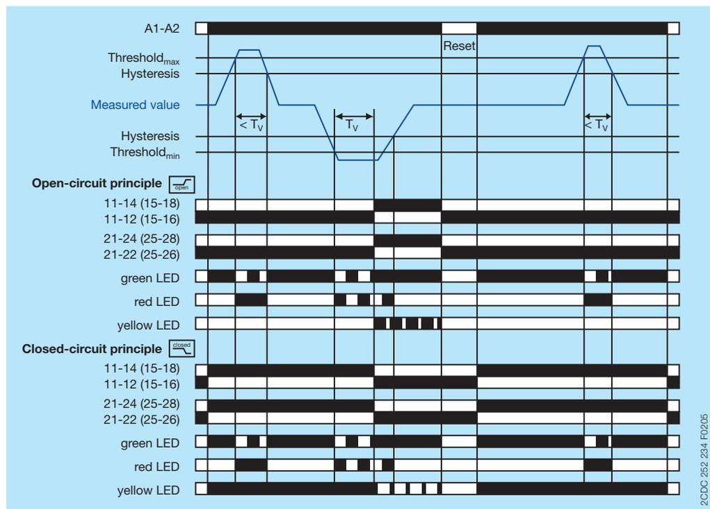
Voltage window monitoring 1x2 c/o (SPDT) contacts  OFF-delayed  with latching
