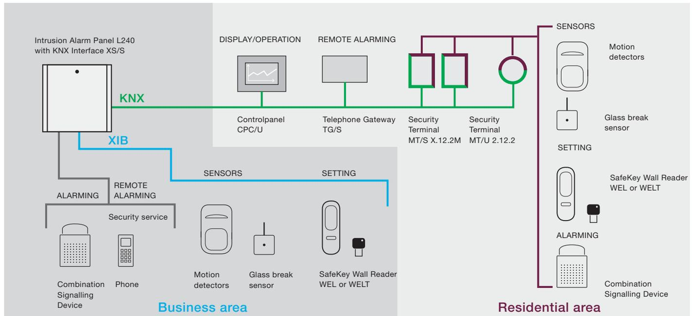
Example of an expansion of the Intrusion Alarm Panel L240 with a KNX Interface XS/S
