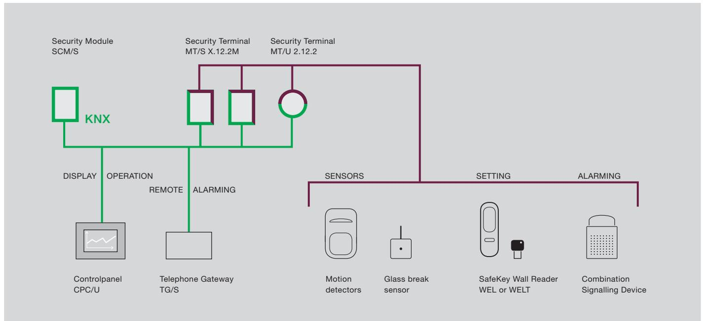
Example of an expansion using Security Module SCM/S
