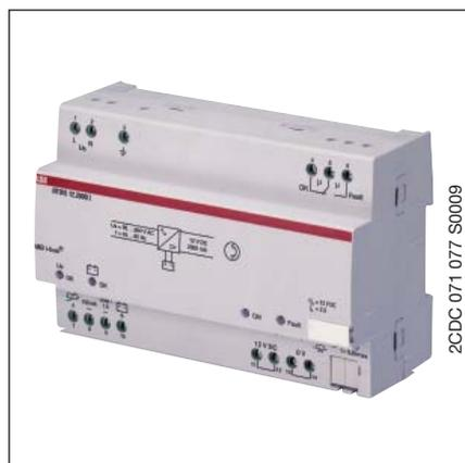
The Uninterruptible Power Supply Unit NTU/S 12.2000.1 is a modular installation device in ProM-Design, for snap-on mounting on a 35 mm mounting rail in a universal, wall-mounted or ceiling panel distribution board as well as in distributed surface mounted housings. The power supply delivers sufficient power for all types of demanding applications with a buffered output voltage of 12 V DC and a maximum output current of 2 A.
