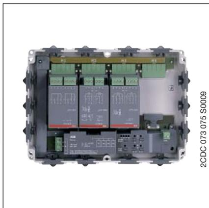
The Room Controller Basis Device RC/A 4.2 can accept up to 4 plug-in modules. It controls their function and communicates as a bus device via the ABB i-bus® KNX.
