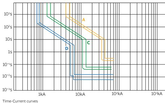
Fig. 2 - Protection thresholds during on-grid operation
