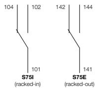
**Withdrawable circuit-breaker with racked-in/racked-out contacts**
