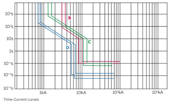
Fig. 3 - Protection thresholds during islanded operation
