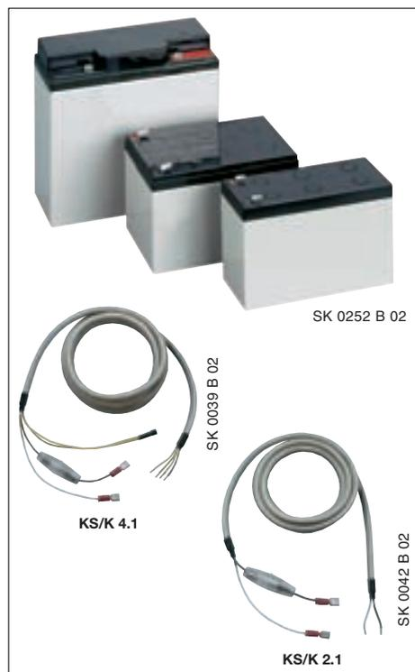
The sealed lead acid batteries SAK7, SAK12 and SAK17 are used to buffer the EIB system voltage in combination with the Uninterruptible EIB Power Supply SU/S 30.640.1. A maximum of 2 batteries can be connected in parallel to the SU/S 30.640.1.
