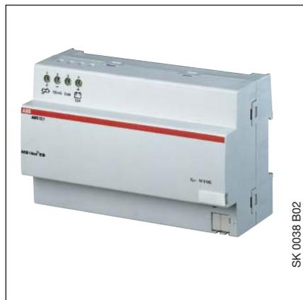
Sealed lead acid battery module for maintaining the ABB i-bus® system voltage (for up to a minimum of 10 minutes) in case of a mains failure in connection with the Uninterruptible EIB Power Supply SU/S 30.640.1. Connection is made via standard cables.
