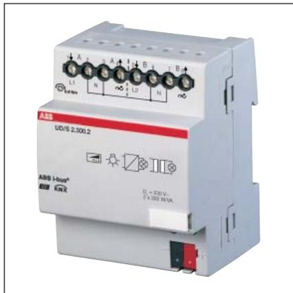
The Universal Dim Actuator UD/S 2.300.2 is a modular installation device (MDRC) for installation in the distribution board. Different load types, e.g. incandescent lamps, 230 V halogen lamps or low-voltage halogen lamps on electronically controlled or conventional transformers, can be connected to two independent outputs.
