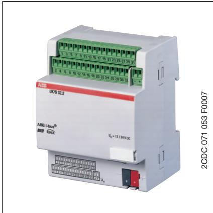
The Universal I/O Concentrator has 32 freely programmable channels, each with a terminal for the connection of floating contacts or signal lamps.
