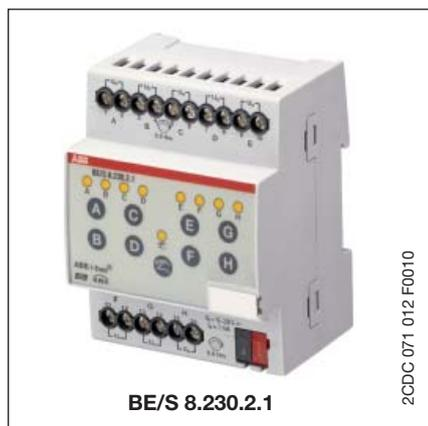
The 8-fold Binary Input BE/S 8.230.2.1 with manual operation is a modular installation device for installation in distribution boards. The device is suitable for detection of 10...230 V AC/DC signals.
