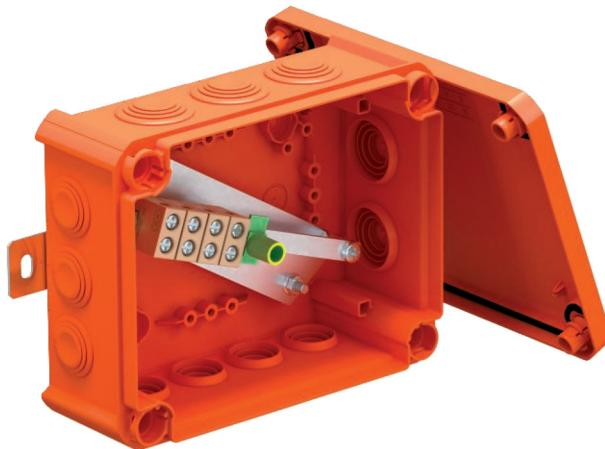
Connection box with soft plug-in seals. Sufficiently large wiring compartment through diagonally-arranged connection unit with completely pre-mounted, high temperature-resistant ceramic terminals. Green and yellow labelled protective conductor terminal. Fastening on easily accessible external flaps. Approved for cable systems that maintain the electrical function according to DIN 4102 Part 12 with the classes E30, E60 and E90.
