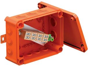
Junction box with ceramic double terminals and soft plug-in seals. Sufficiently large wiring compartment through diagonally-arranged connection unit with completely pre-mounted, high temperature-resistant ceramic terminals. Green and yellow labelled protective conductor terminal. Fastening on easily accessible external flaps. Approved for cable systems that maintain the electrical function according to DIN 4102 Part 12 with the classes E30, E60 and E90.
