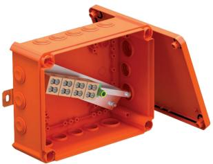
Junction box with ceramic double terminals and soft plug-in seals. Sufficiently large wiring compartment through diagonally-arranged connection unit with completely pre-mounted, high temperature-resistant ceramic terminals. Green and yellow labelled protective conductor terminal. Fastening on easily accessible external flaps. Approved for cable systems that maintain the electrical function according to DIN 4102 Part 12 with the classes E30, E60 and E90.
