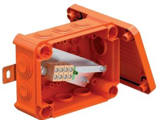
Connection box for data technology with soft plug-in seals. Pairs of high temperature-resistant ceramic terminals, suitable for data cables. Green and yellow labelled protective conductor/shield terminal. Fastening on easily accessible external flaps. Approved for cable systems with electrical function maintenance according to DIN 4102 Part 12 with the classes E30, E60 and E90.
