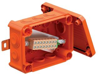
Connection box for data technology with soft plug-in seals. Pairs of high-temperature-resistant ceramic terminals, suitable for data cables. Green-yellow labelled protective conductor/shield terminal. Fastening on easily accessible external flaps. Approved for cable systems that maintain the electrical function according to DIN 4102 Part 12 with the classes E30, E60 and E90. Including 2x MMSplus P 6x35 screw ties.
