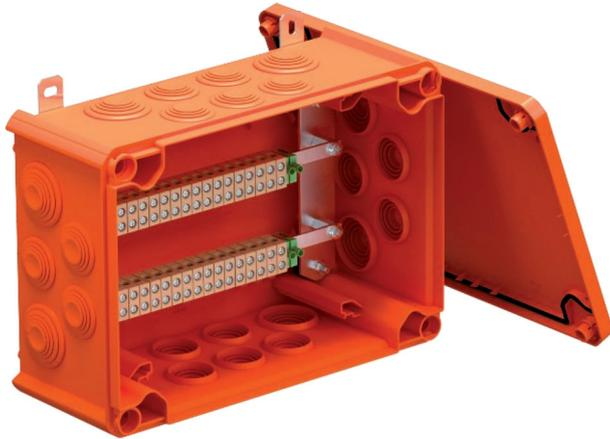
Connection box for data technology with soft plug-in seals. Pairs of high-temperature-resistant ceramic terminals, suitable for data cables. Green-yellow labelled protective conductor/shield terminal. Fastening on easily accessible external flaps. Approved for cable systems that maintain the electrical function according to DIN 4102 Part 12 with the classes E30, E60 and E90. Including 2x MMSplus P 6x35 screw ties.
