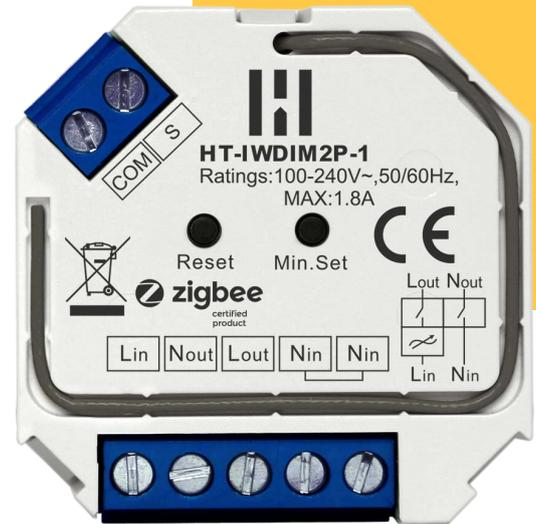
Trailing edge built-in smart dimmer. Control your lights locally from your existing switch, or from anywhere by the app when connected to your Heimgard smart home system. This product does not work in combination with wireless smart LED bulbs!
