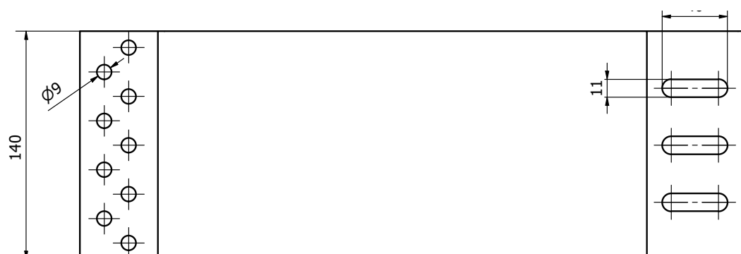
Fig. 2 Dimensions of the K-44 element - top view.
