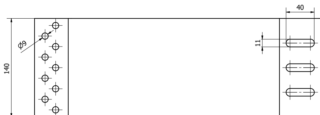
Fig. 3 Dimensions of the K-44-W element - side view
