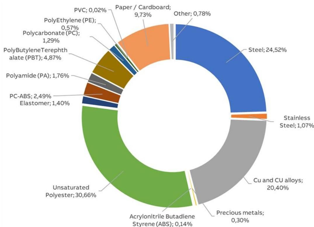
Figure 1: Composition of XT3 3p IEC C-N-S TMD 250A
