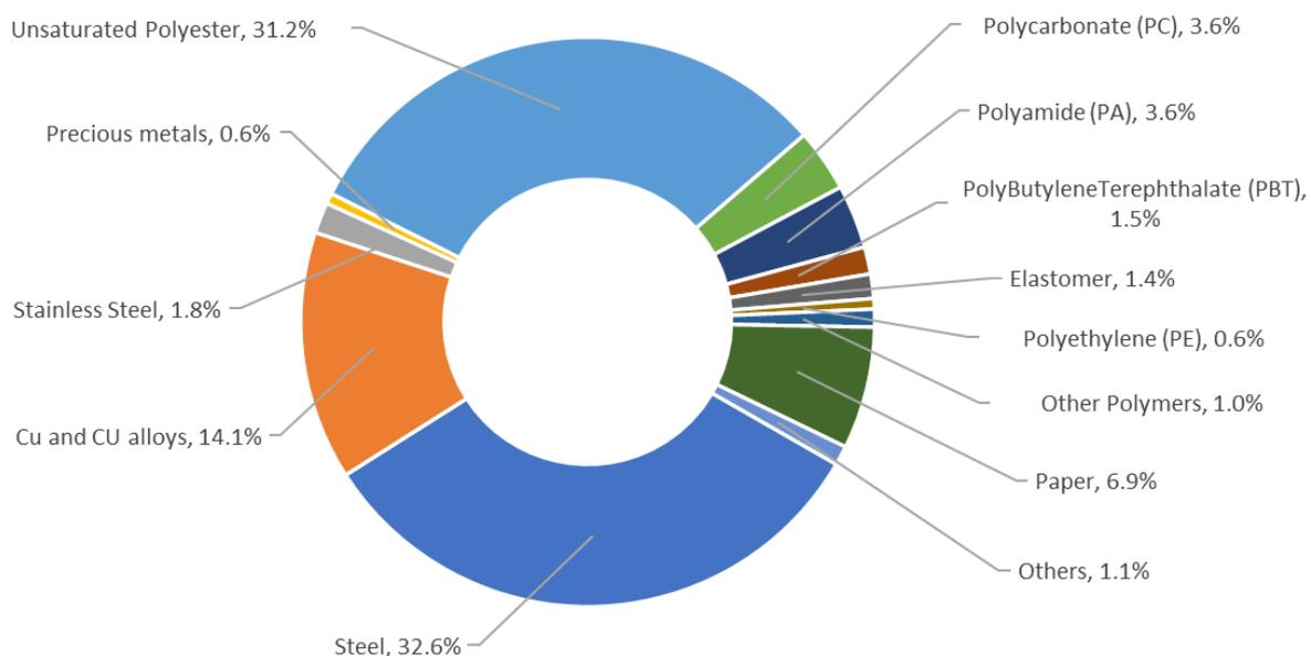
Figure 1: Composition of XT4 IEC-3P-N-S-H-L-TMA 250A
