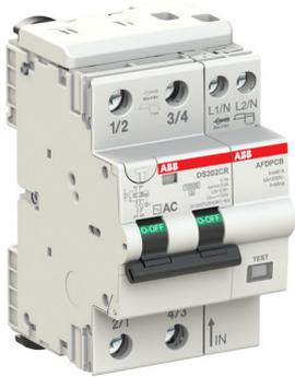
AFD unit AFDPCB can be combined with 2P RCBO in 2M of DS202CR series providing protection up to 40A against overcurrents, residual currents and arc faults currents. Perfect solution in 3M for a complete protection in two phases applications. Signal and auxiliary contacts can be added on the left side of DS202CR.
