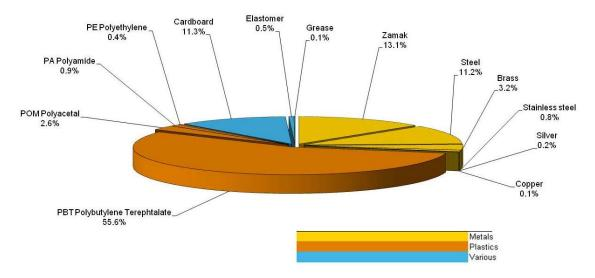
The total mass of XCKS131 and of its installation components (the assumption is made that four M5 hexagon socket cap screws are used) is 208 g and the materials are distributed as follows:
