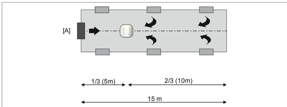
Fig. 17: Positioning example of a dead-end hallway smoke section with one door
