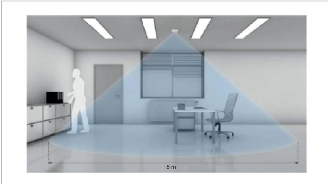
Fig. 6: Outer detection range (using Busch-Presence detector Mini KNX as an example)
