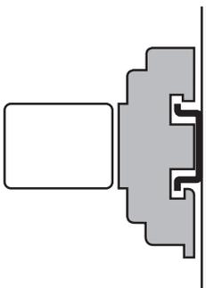
• Use two M3 screws to mount the case-surface mounting (MY□F) and tighten them securely. (Appropriate tightening torque: 0.98 N·m)
