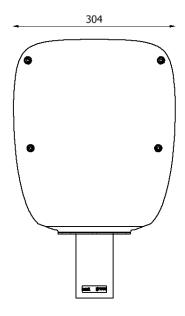
**Next Green Poleplate** is a charger mount for installation on a  $\emptyset$  60 mm pole. Poleplate is made of Swedish steel and powder coated to provide the highest durability and quality. Poleplate enables easy mounting of a charging box to a steel tube.
