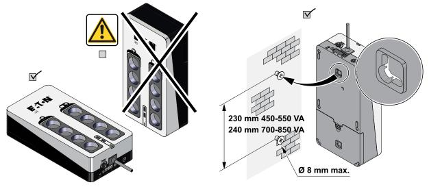
For 3S450 and 3S550 only do not dispose the product on the side as shown below.
