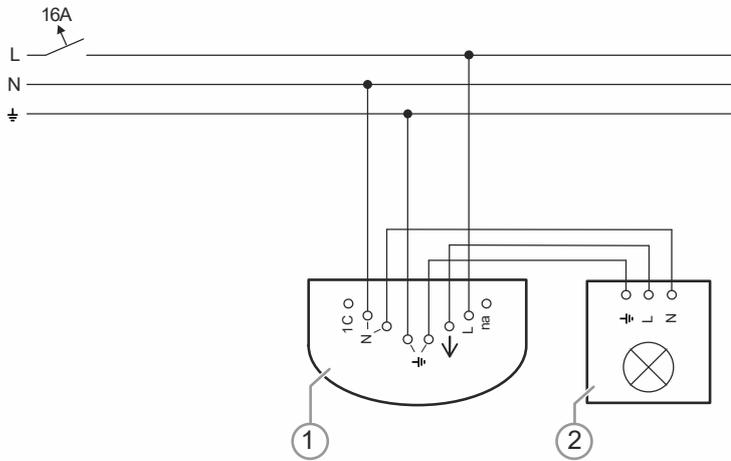
Fig. 23: Examples of switching: Single offices light control without extension unit input
