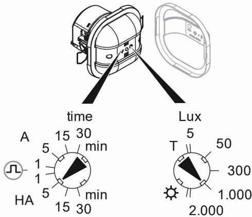
Fig. 6: Setting via trimmers
