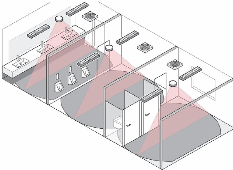
Fig. 37: Application example: DALI in a simple WC facility
