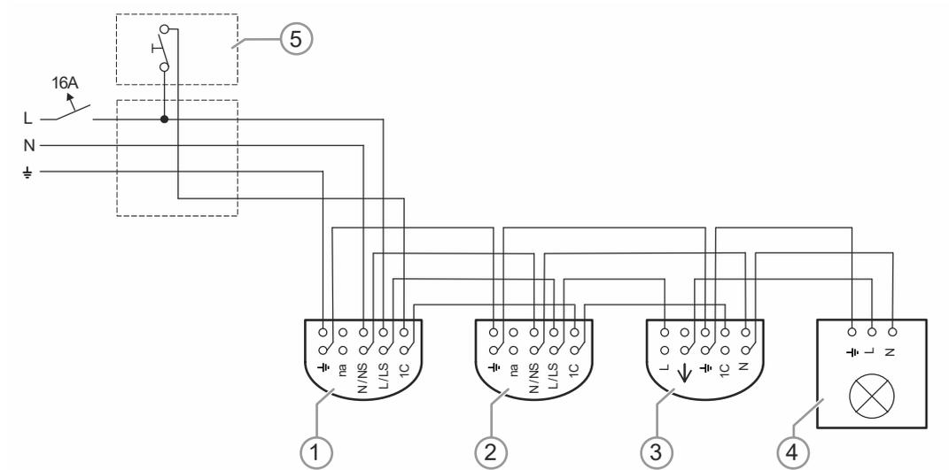
Fig. 52: Examples of switching: corridor (main unit/extension unit) light control with extension unit input
