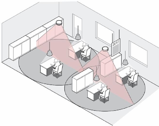
Fig. 62: Sources of interference: heat sources without interference effect
