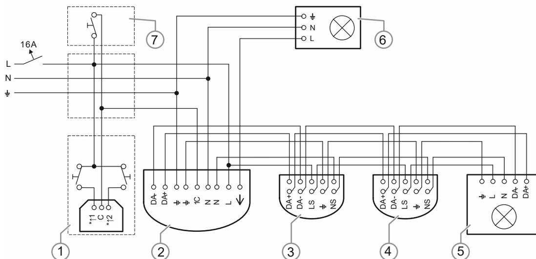
Fig. 28: Examples of switching: DALI light control with extension unit input and blackboard light in classroom
