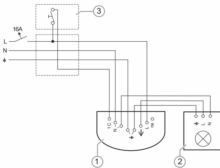
Fig. 57: Examples of switching: light control with extension unit input and moisture-protected device at a private house
