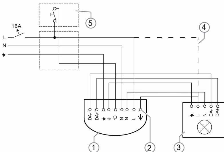
Fig. 38: Examples of switching: DALI light control with extension unit input for simple WC facility
