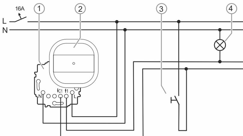
Fig. 49: Examples of switching: corridor light control with extension unit input
