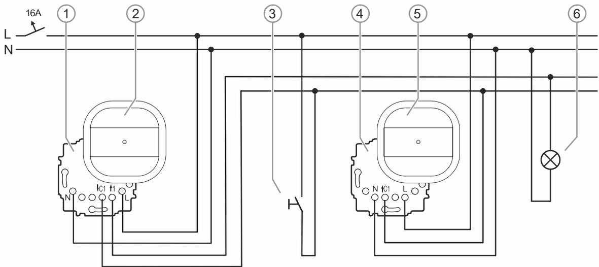
Fig. 53: Examples of switching: stairwell (main unit/extension unit) light control with extension unit input
