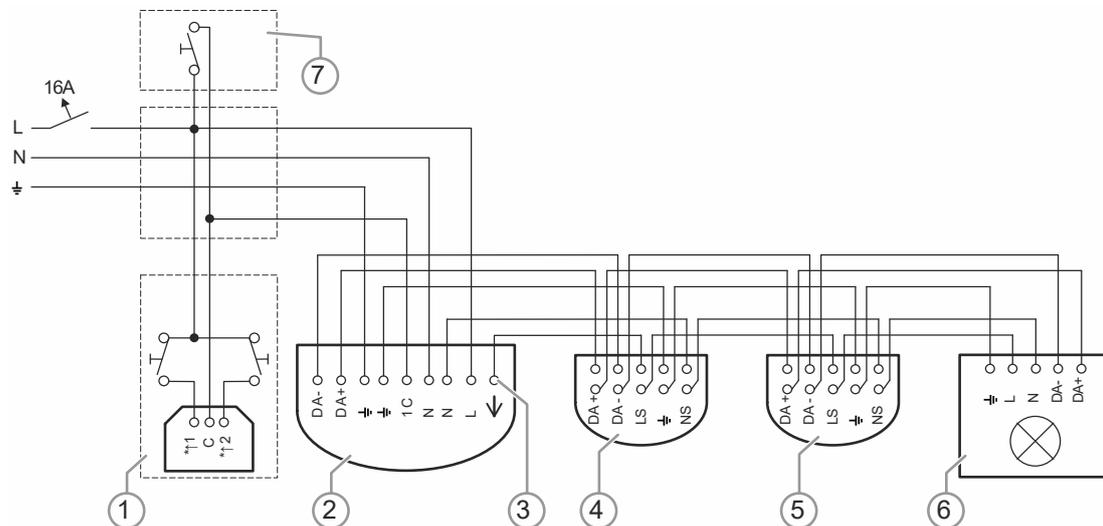
Fig. 42: Examples of switching: DALI daylight-dependent control (main unit/ extension unit) with extension unit input
