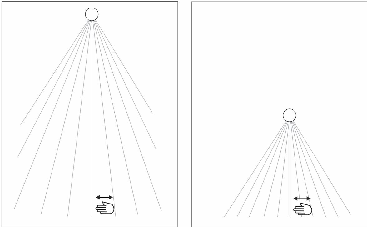
Fig. 21: Mounting heights (presence detector)
