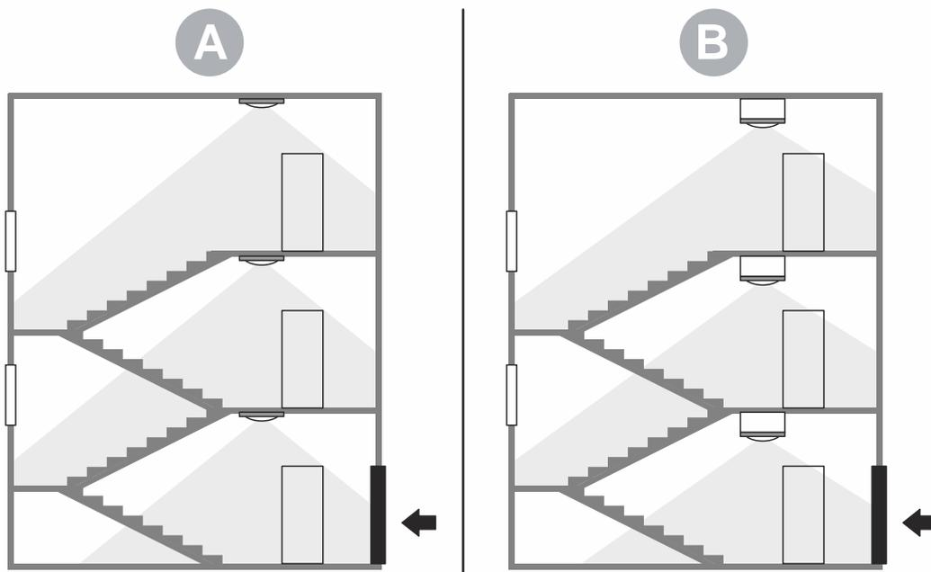
Fig. 51: Application example: stairwell with one main entrance
