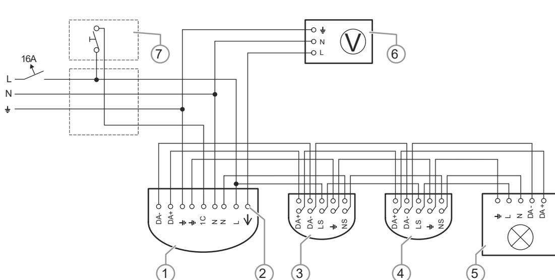
Fig. 39: Examples of switching: DALI light control (main units/extension units) with extension unit input and fa control for WC facility
