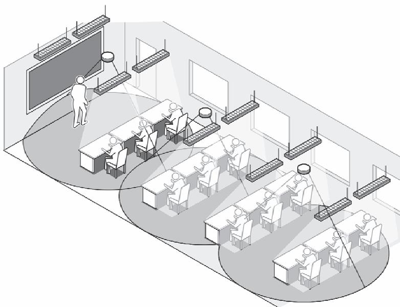
Fig. 29: Application example: classroom with blackboard light and daylight-dependent control
