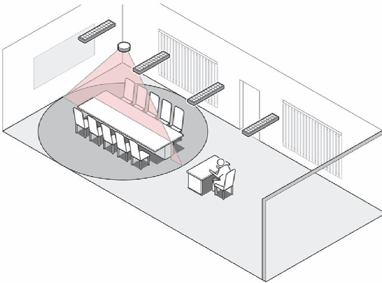
Fig. 40: Application example: daylight-dependent control
