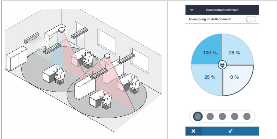
Fig. 63: Sources of interference: remedy
