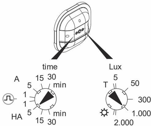
Fig. 9: Setting via trimmers
