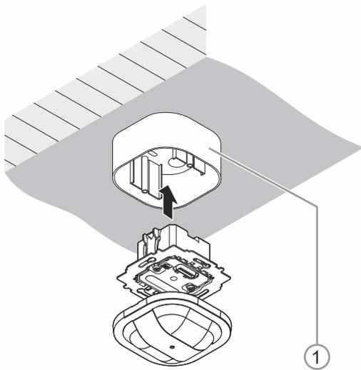
Fig. 5: Surface mounting ABB flexTronics®
