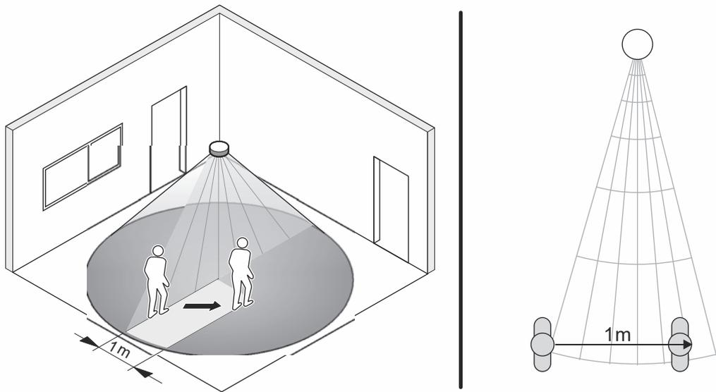
Fig. 19: Detection crosswise to the device
