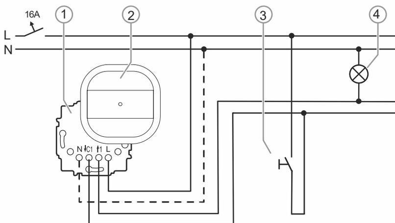
Fig. 26: Examples of switching: Single offices light control with extension unit input
