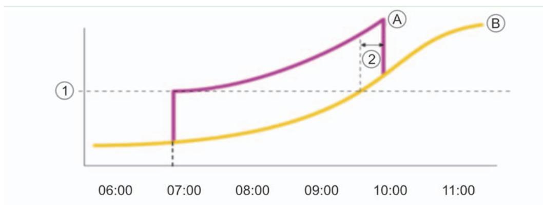
Fig. 43: Control for constant light switch function
