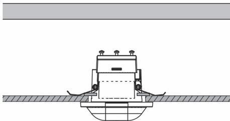
Fig. 3: Mounting situation: suspended ceiling
