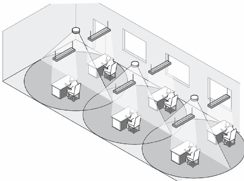
Fig. 35: Application example: DALI in an open-plan office
