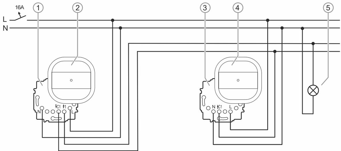
Fig. 55: Examples of switching: gymnasium (main unit/extension unit)
