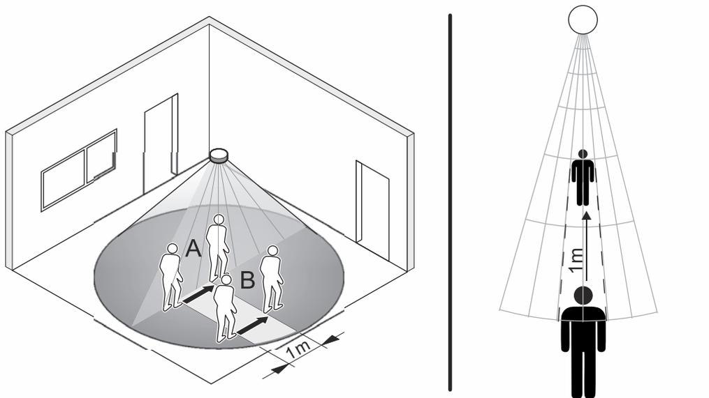
Fig. 20: Moving lengthways / parallel to the device
