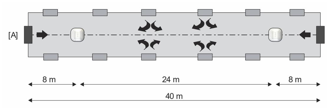
Fig. 46: Application example: escape route corridor with two doors (fire sector)
