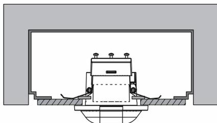
Fig. 4: Mounting situation: concrete slab
