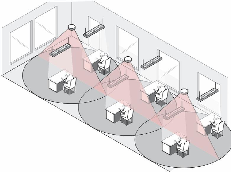
Fig. 58: Application example: open-plan office with illuminated glass front
