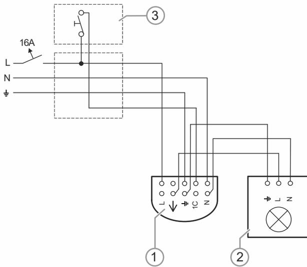
Fig. 47: Examples of switching: corridor light control with extension unit input
