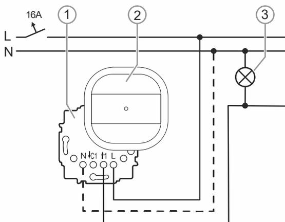
Fig. 25: Examples of switching: Single offices light control without extension unit input
