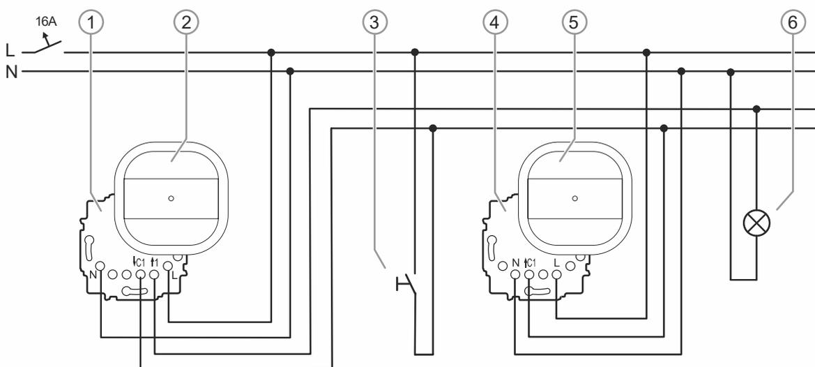
Fig. 50: Examples of switching: corridor (main unit/extension unit) light control with extension unit input
