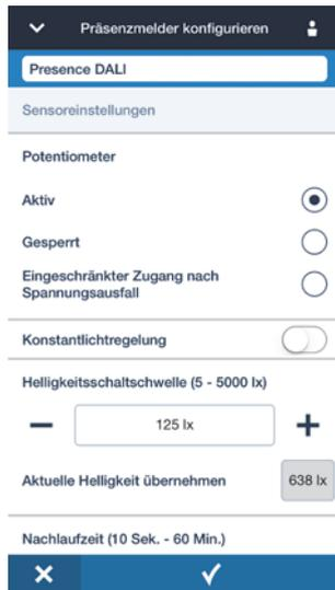
Fig. 41: Adaptation of the brightness set value for the daylight-dependent control
