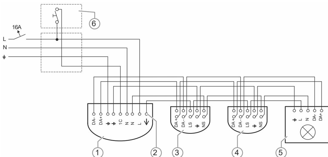
Fig. 59: Examples of switching: DALI light control system with extension unit input and basic lighting in a larger office
