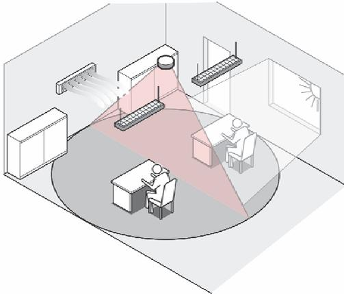
Fig. 61: Sources of interference: external heat sources
