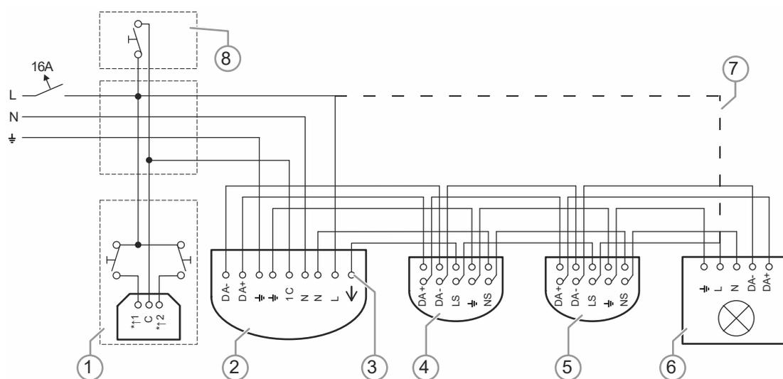
Fig. 36: Examples of switching: Open-plan office (main unit/extension unit) DALI light control with extension unit input
