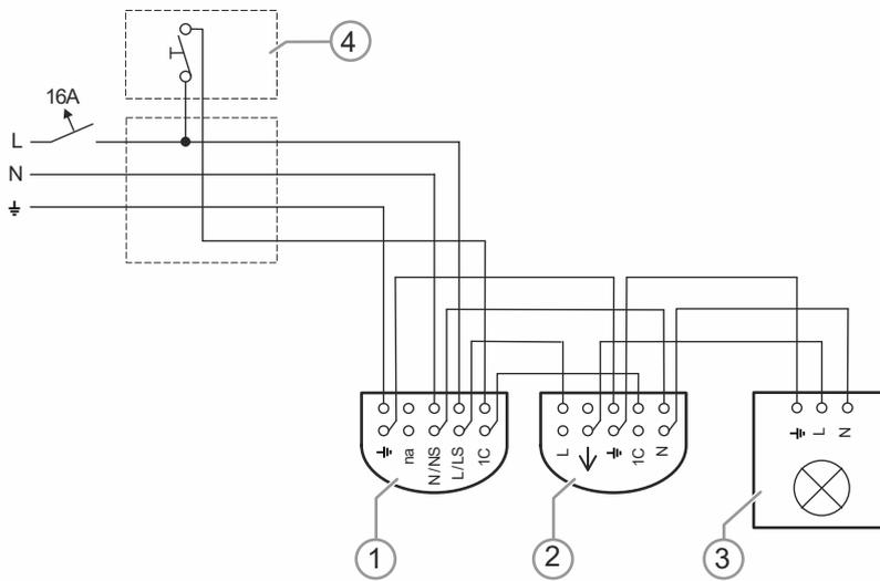
Fig. 48: Examples of switching: corridor (main unit/extension unit) light control with extension unit input
