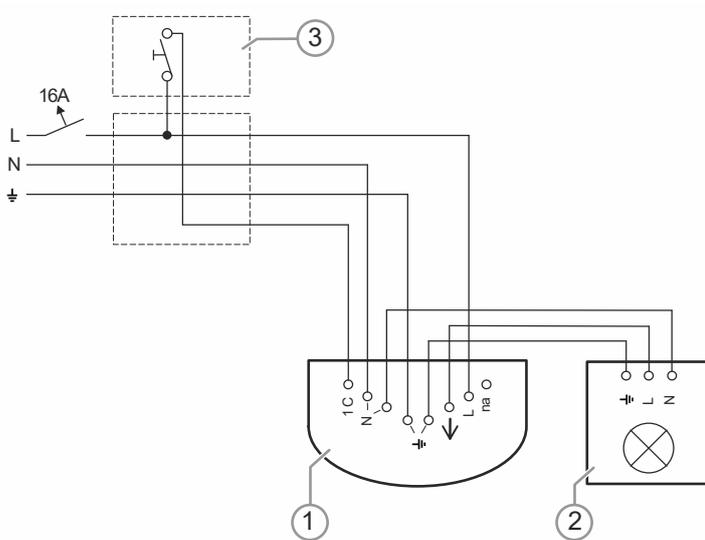
Fig. 24: Examples of switching: Single offices light control with extension unit input
