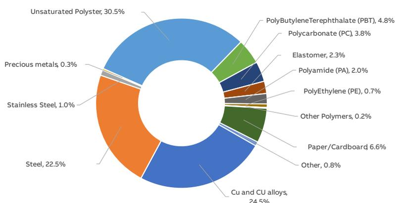
Figure 1: Composition of XT3 250 N 3P IEC TMD
