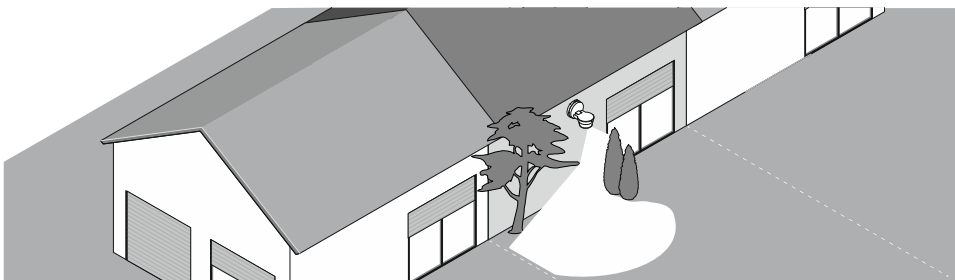
Fig. 23: Wall mounting on centre-row house for limited detection radius 6851/9-xxx
