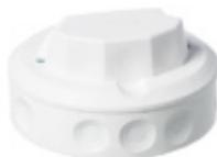
The round, dual-component connection box AP7.1 (2,5 mm<sup>2</sup>, 400 V, IP44) is equipped with 10 membrane cable entries (17 mm) and two in the bottom. The cover of the box is equipped with three membrane seals (one Ø20 mm and two Ø16 mm) and with three strain-reliefs.
