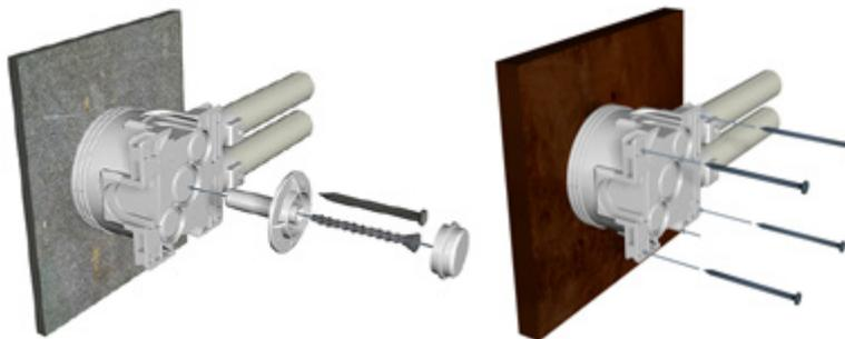
Installation plug AS25 is used together with a screw or a nail to fasten boxes to a casting mould through the center knockout in the bottom. When the mould is disassembled, the screw or nail will follow the plywood mould and does not have to be separately removed.
