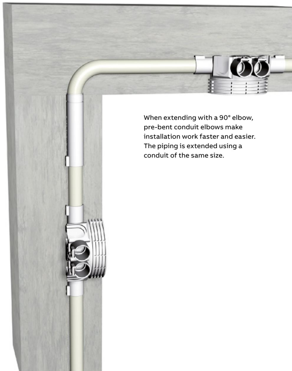
When extending with a 90° elbow, pre-bent conduit elbows make installation work faster and easier. The piping is extended using a conduit of the same size.
