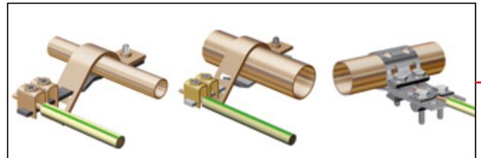
The AM11 earthing terminal is used, for example, for the potential equalization of air-conditioning and ventilation ducts. The earthing terminal is affixed using two pull rivets (pop-rivets) c/c 3,2 mm to the surface of the duct. The terminal bar is made of tinned copper and has a single <math><10\text{ mm}^2\text{ Cu}</math> terminal.
