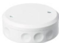
The round junction box AP7 (2,5 mm<sup>2</sup>, 400 V, IP44) is similar to the AP9 and the AP10 is equipped with 10 membrane cable entries (Ø17 mm) at the sides and two in the bottom. Cables are easy to connect by simply inserting the stripped ends through the inlets. The cover is locked with two screws at distance of 78 mm. The box can be furnished with strain-reliefs AS9, AS9.1 and AS9.3. Made of halogen free material (IEC/61249-2-21).
