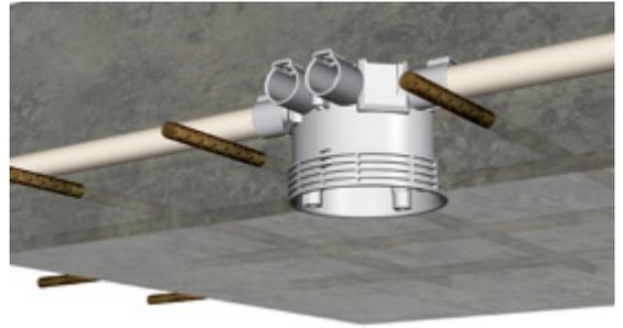
The overall height of the box is 73 mm which gives plenty of connecting space. The height from the conduit to the edge of the box is 47 mm. It is sufficient for the installation of piping above the reinforcements, without difficult and time-consuming extra work.
