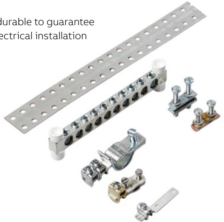
The AM8 earthing terminal is mainly used for connecting the earthing conductors to various pipework. Due to the structure of the terminal, it is possible to adjust it to suit to four different pipe thicknesses between 8 to 28 mm. The terminal has two 35 mm<sup>2</sup> pillar terminals. The conductor bar is made of tinned copper and the strap of zinc-plated steel.
