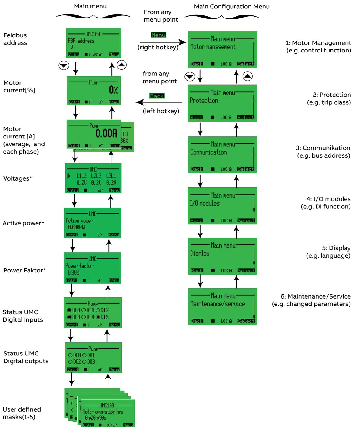
With the right soft key **Select** you can enter the selected submenus which are described in the following sections. The masks shown with a star \* are only displayed if the voltage module is present.
