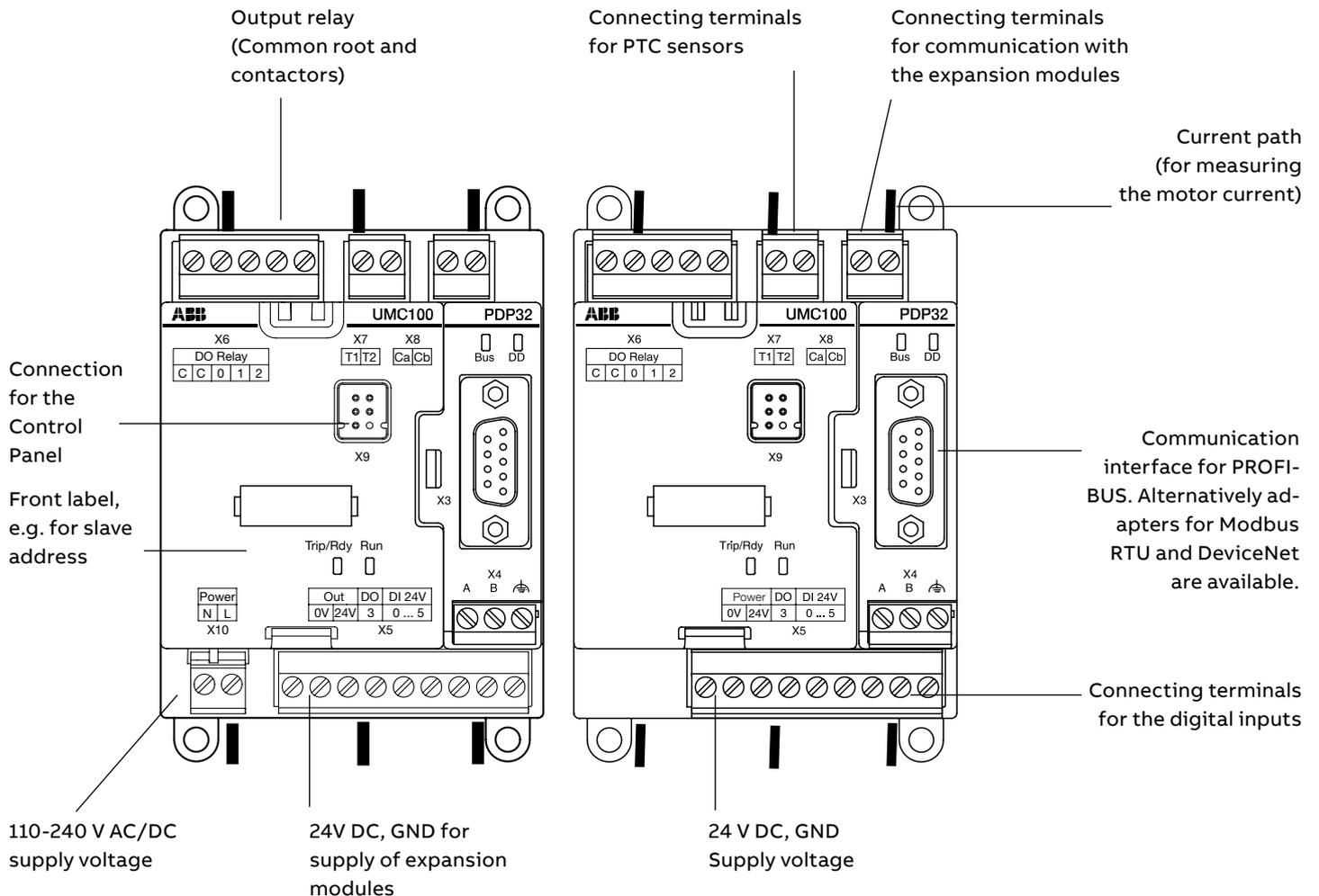
After powering on, the UMC100.3 performs a self-test of its hardware and checks the configuration for consistency. In the event of a failure, a self-test fault is generated and signalled. Replace the device in such a case. After a successful self-test the UMC enters the operational state.
