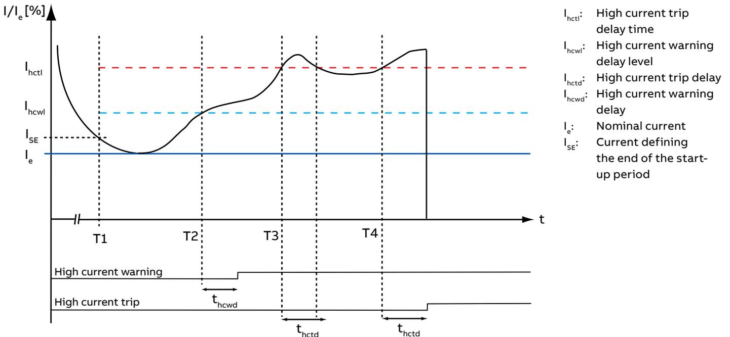
**Trend diagram of the motor current over time**
