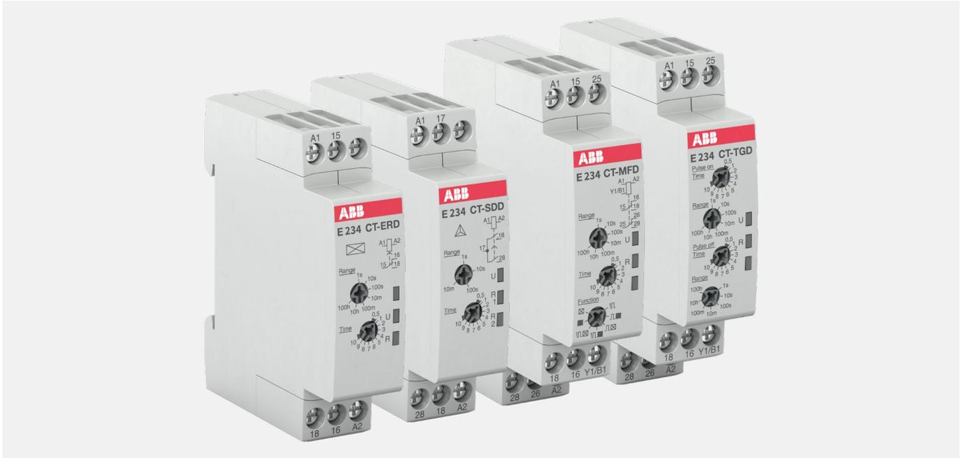
The CT-D range is ideal for building applications and installation panels, due to its compact modular housing. For maximum flexibility in operation, nine single-function as well as two multifunction devices with seven timing functions are available. The devices offer four or seven time ranges from 0.05 seconds up to 100 hours. Their wide supply voltage range allows their use in applications worldwide.
