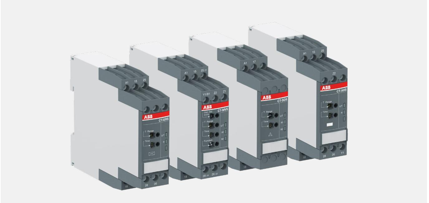
The advanced CT-S range includes 22 single-function devices and 16 multifunction timers with up to 13 functions. The devices feature seven or ten time ranges, which are adjustable from 0.05 seconds to 300 hours. Every device is available in two different connection technologies: double-chamber cage connection terminals or ABB's vibration-resistant Push-in Technology.
