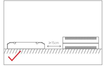
Please do not place the products on LED drivers. The distance between the product and the driver should be  $\geq 15\text{cm}$  so as not to affect heat dissipation and shorten the lifespan of the products.
