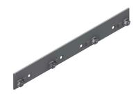
**Additional information:** Two splice connectors required for each connection. It is the recommended splice connector for cable trays in SS. 2 splice connectors are used for each joint. An additional Splice Plate is recommended for tray widths over 300 mm.
