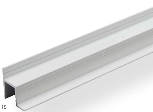
Our profile for ceiling-to-wall mounting creates a decorative grazing light along the wall surface and is available in white, black, and aluminium. An opal cover lid provides a softer, more even light without visible diodes – perfect for applications like wall lighting. A clear cover lid gives a more direct light with higher output, ideal for functional lighting in shelves or workspaces. This solution offers both aesthetics and functionality, making it an excellent choice for creating ambience.
