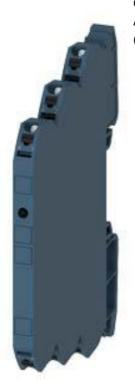
Output coupler 1 CO contact hard gold-plated 24 V AC/DC Enclosure width 6.2 mm Spring-load. terminal (push-in) Thermal current 6 A
