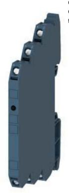
Output coupler Optocoupler 1 NO, transistor, 24 V DC Output max. 30 V DC, 2 A short circuit-proof Screw terminal Overall width 6.2 mm Thermal current 2 A
