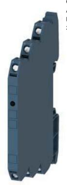
Output coupler Optocoupler 1 NO transistor, 110-230V AC/DC Output max. 30 V DC, 3 A short circuit-proof Enclosure width 6.2 mm Screw terminal Thermal current 3 A
