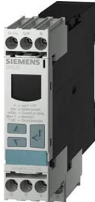
DIGITAL MONITORING RELAY COS-PHI A. CURRENT MONITORING FROM 90 TO 690V AC OVERSHOOT AND UNDERSHOOT INTERNAL POWER SUPPLY AC 50 TO 60 HZ SPIKE DELAY 0.1 TO 20S HYSTERESIS W. (I) 0.1 TO 2A 2 CHANGEOVER CONTACTS W. OR W/O ERROR LOG SCREW TERMINAL REPLACEMENT PRODUCT F. 3UG3014
