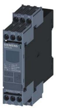
DIGITAL MONITORING RELAY COS-PHI AND CURRENT MONITORING FOR IO-LINK 90 TO 690V AC, 0.2 TO 10A OVERSHOOT AND UNDERSHOOT ON DELAY TIME TRIPPING DELAY TIME HYSTERESIS 0.1 TO 3.0A 2 CHANGE-OVER CONTACTS, SCREW TERMINAL
