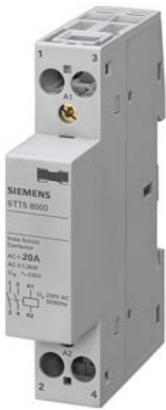
INSTA CONTACTOR WITH 1 MAKE AND 1 BREAK CONTACT CONTACT FOR 230, 400 V AC, 20 A TRIGGERING 24 V AC
