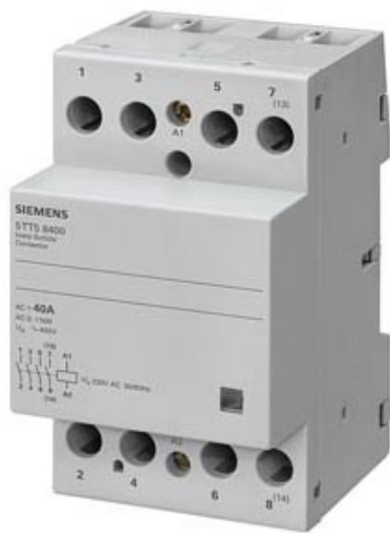
INSTA CONTACTOR WITH 2 MAKE A. 2 BREAK CONTACTS CONTACT FOR 230, 400 V AC, 40 A TRIGGERING 24 V AC
