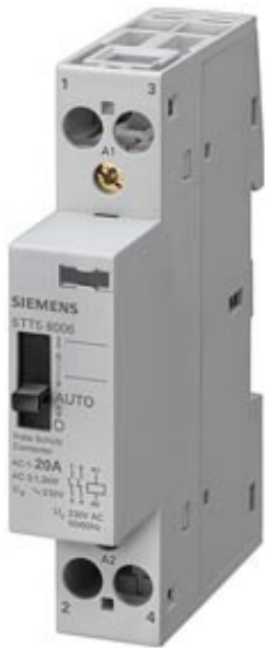
INSTA CONTACTOR 0/1 AUTOMATIC WITH 1 MAKE AND 1 BREAK CONTACT CONTACT FOR 230, 400 V AC, 20 A TRIGGERING 24 V AC
