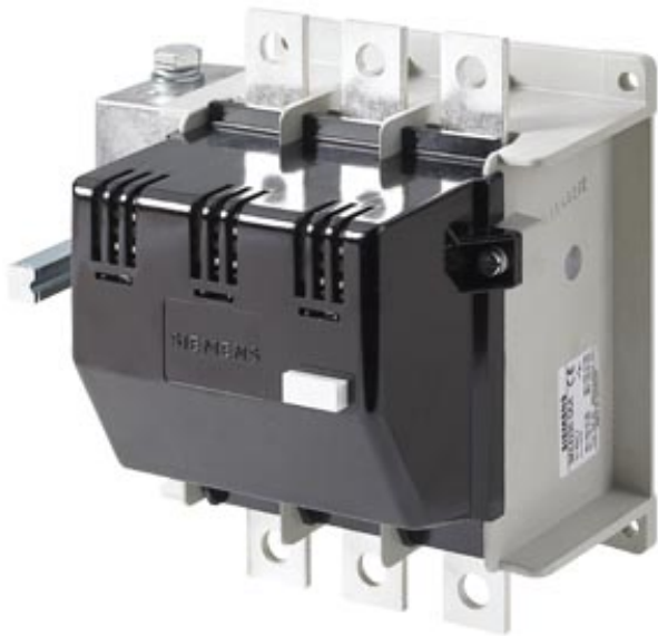
SWITCH DISCONNECTOR 3-POLE I=1000A, U=690V, FRONT ROTARY OPERATING MECHANISM WITHOUT HANDLE
