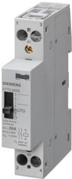
INSTA CONTACTOR 0/1 AUTOMATIC WITH 1 MAKE AND 1 BREAK CONTACT CONTACT FOR 230, 400 V AC, 20 A TRIGGERING 230 V AC
